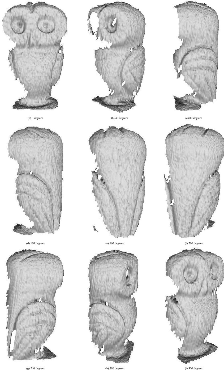
Figure 7: This figure shows nine range images of a small owl figurine seen from nine different viewpoints. The views were obtained by rotating the object on a precision turntable by 40 degree intervals. The views shown above were pre-processed in order to remove spurious data points and background surfaces, such as the platform of the turntable on which the object was resting, so that only the owl's surface remained.
